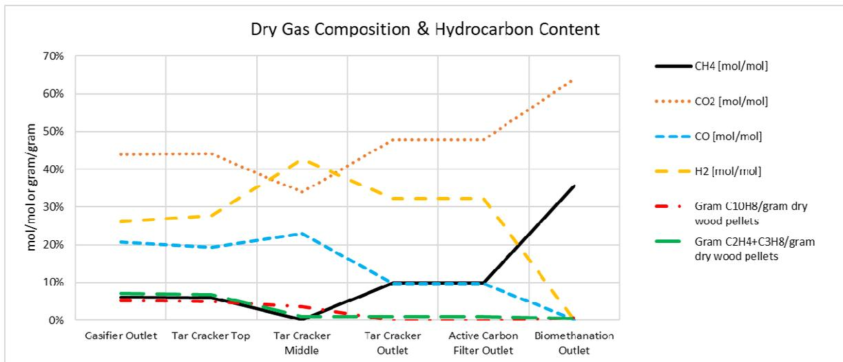
Figure 3. The composition of the main components throughout the total reactor system
