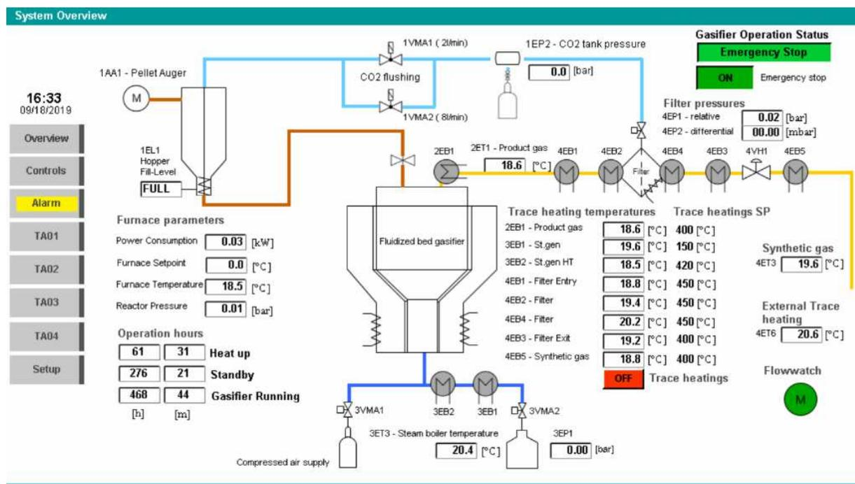
Figure 1. System overview of the gasifier (not in operation)
