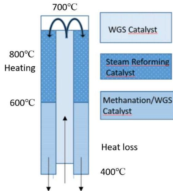
Figure 2. Steam reforming and pre-methanation unit; the tar cracker
