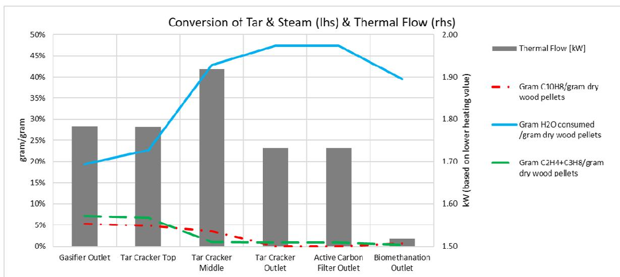
Figure 4. The steam consumption, tar reduction and energy content in the gas flow
